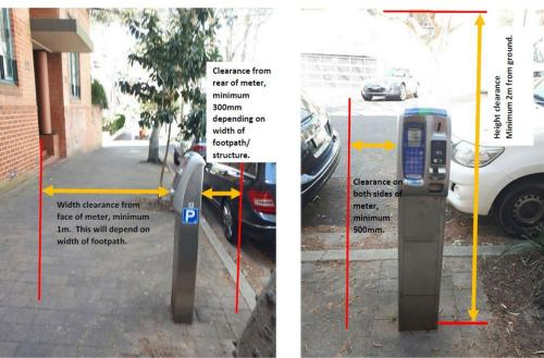
Figure: Parking Meter - clearance details, for hoarding or other structures
