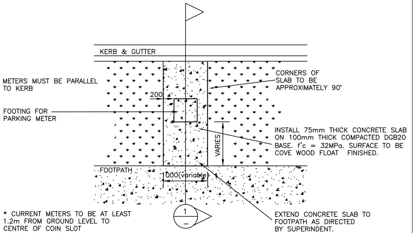
\* CURRENT METERS TO BE AT LEAST 1.2m FROM GROUND LEVEL TO CENTRE OF COIN SLOT
