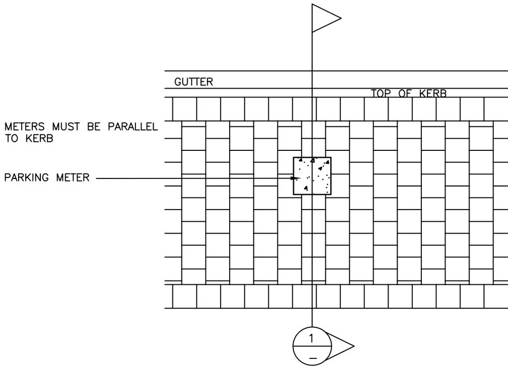
\* CURRENT METERS TO BE AT LEAST 1.2m FROM GROUND LEVEL TO CENTRE OF COIN SLOT
