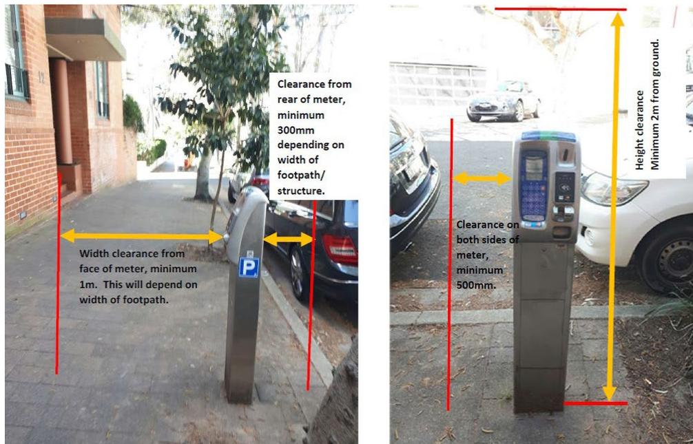
**Figure:** Parking Meter – clearance details, for hoarding or other structures
