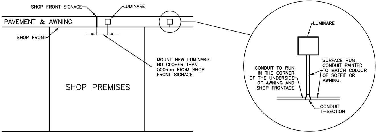
LUMINARE MOUNTING POSITION DETAIL
