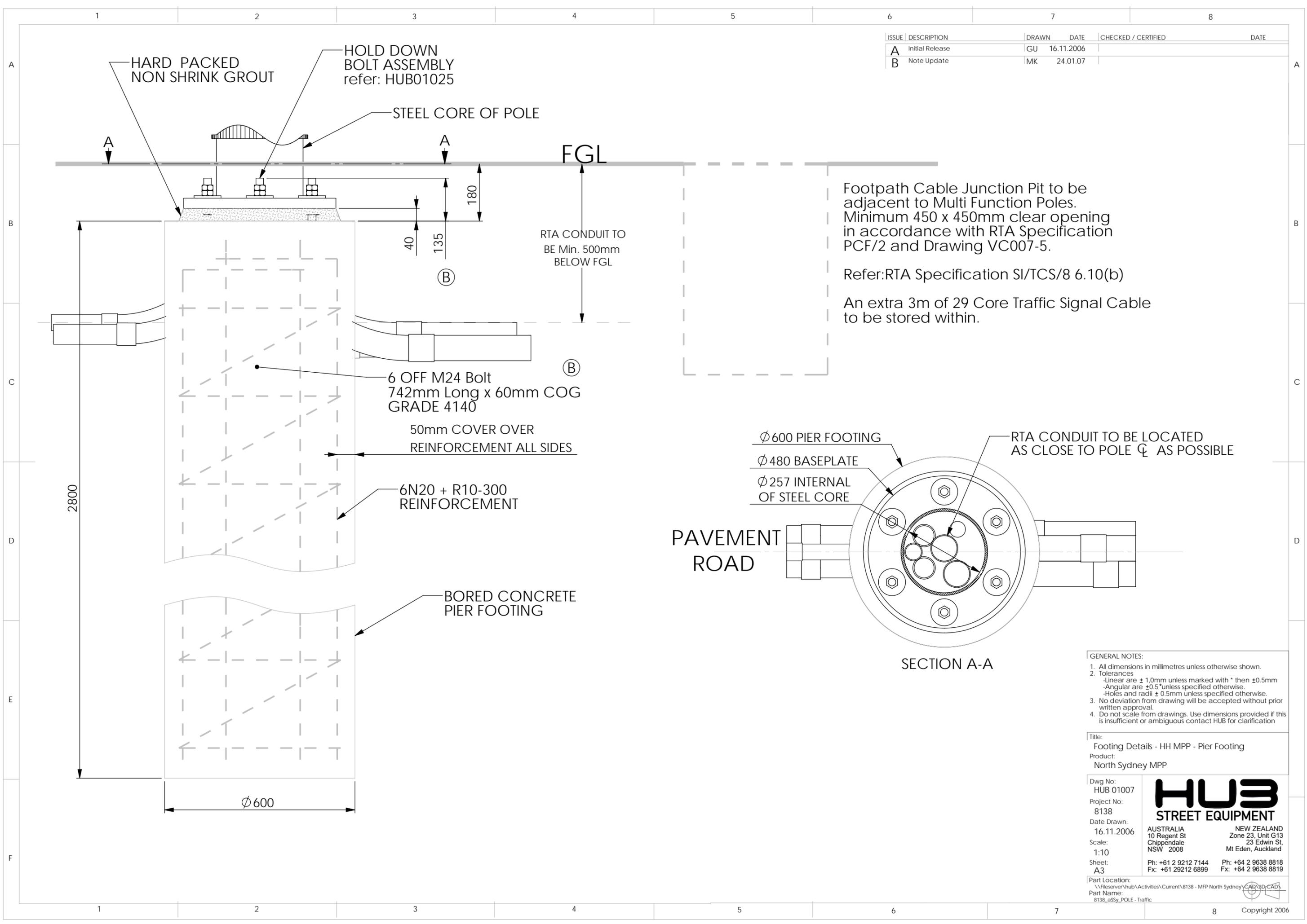
Footpath Cable Junction Pit to be adjacent to Multi Function Poles. Minimum 450 x 450mm clear opening in accordance with RTA Specification PCF/2 and Drawing VC007-5.
