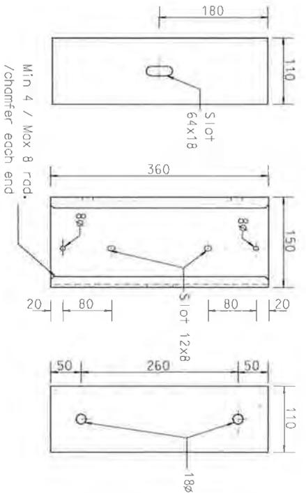
BLOCKOUT PIECE - W BEAM (P002)
