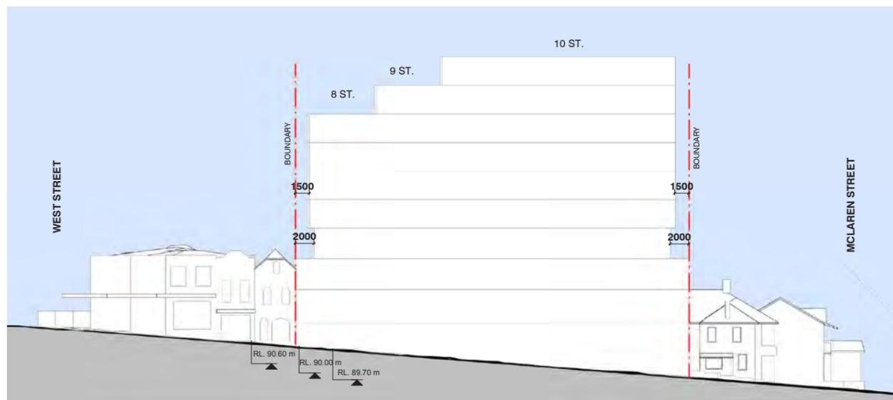
Figure 28. Tower envelope - Option 1 (source: PTW).
