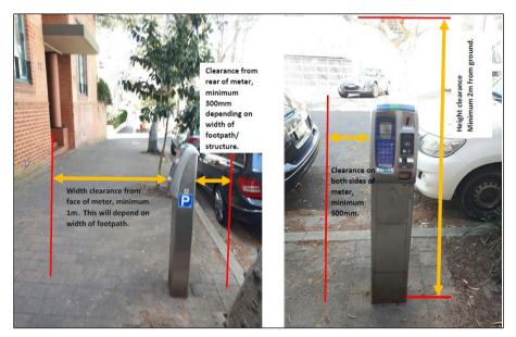
Figure 5: Parking Meter - clearance details, for hoarding or other structures
