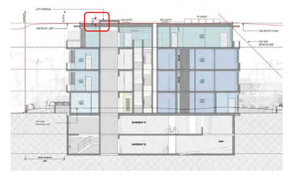
Figure 4 Section (2) illustrating height non-compliance
