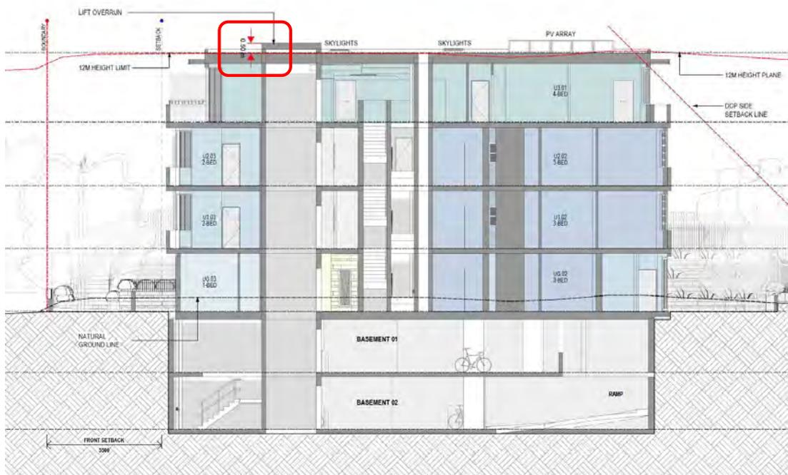
Figure 4 Section (2) illustrating height non-compliance
