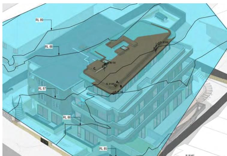
Figure 33. Height Plane Diagram indicating the extent of the proposed variations
