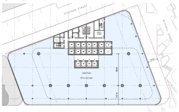
Figure 11 Typical Podium Floor Plate
