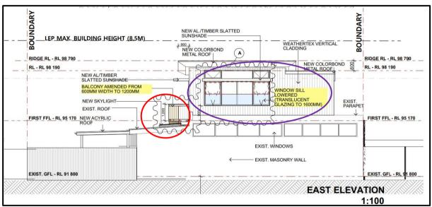
Figure 1: Proposed east elevation showing changes to balcony (circled in red) and windows (circled in purple) in master bedroom (first floor)
