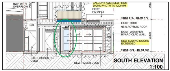
Figure 4: Proposed south elevation – additional sliding door incorporated in area (circled in green)
