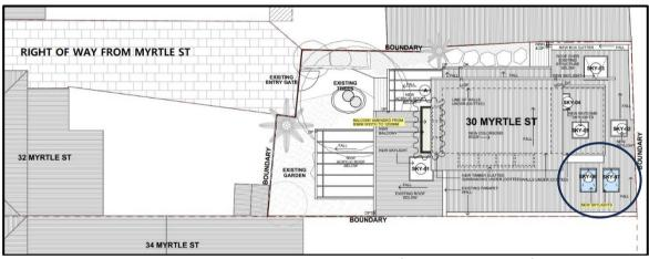
Figure 5: Site plan showing new skylights (circled in dark blue)
