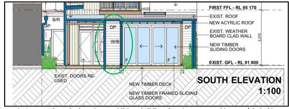
Figure 3: Approved south elevation – additional sliding door incorporated in area (circled in green)
