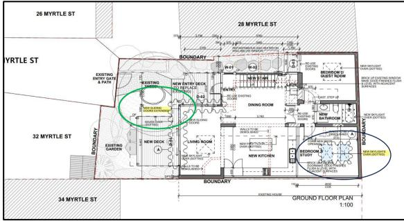
Figure 6: Ground floor plan showing additional sliding door (circled in green) and new skylights (circled in dark blue)
