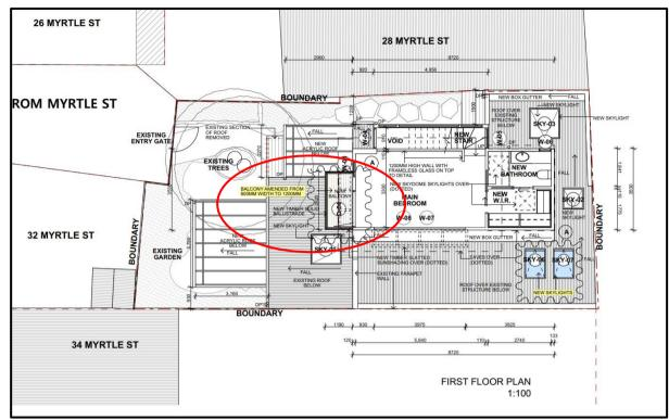
Figure 2: Proposed first floor plan showing balcony extending from 0.6m to 1.2m (in depth) (circled in red)
