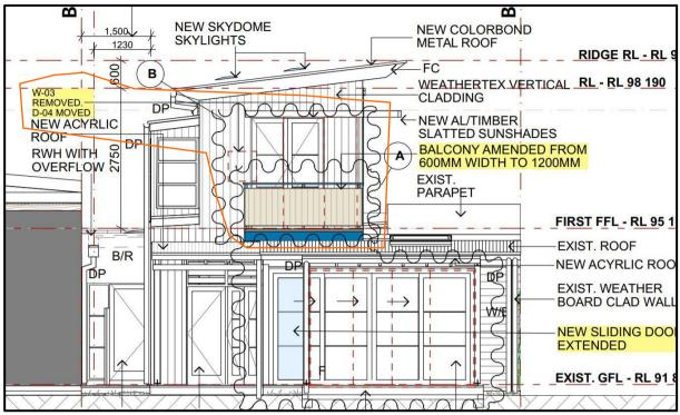
Figure 7: South elevation showing deletion of window and relocated balcony door (outlined in orange)
