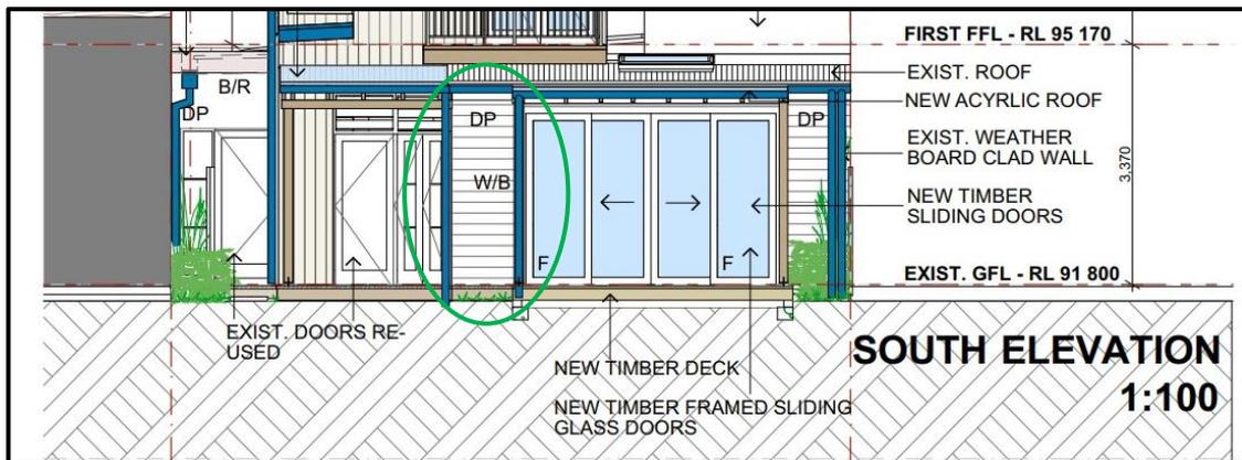
Figure 3: Approved south elevation – additional sliding door incorporated in area (circled in green)
