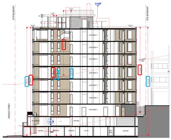
Figure 3 Section illustrating maximum height non-compliance (Blue indicates height from existing floor level, red indicates height from extrapolated topography)
