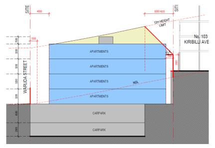
Figure 7 Compliant envelope scheme
