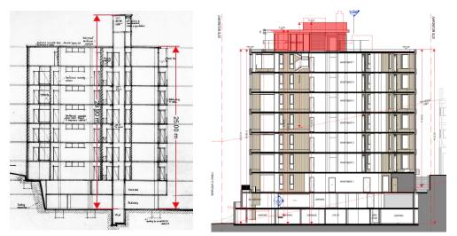
Figure 5 Existing section (left), proposed section (right), with new components highlighted red
