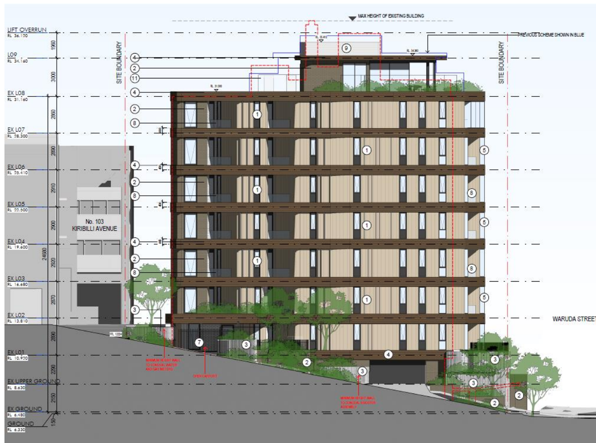
Figure 6: Western elevation showing pedestrian and vehicular access to the carport (left) and the upper ground parking level from Beulah Street, and an indication of proposed landscaping. Also shown in both drawings is linework to compare the existing building envelope (red dotted line), the originally submitted design (blue outline, for changes to roof only), and the current design (Nettleton Tribe Architects).
