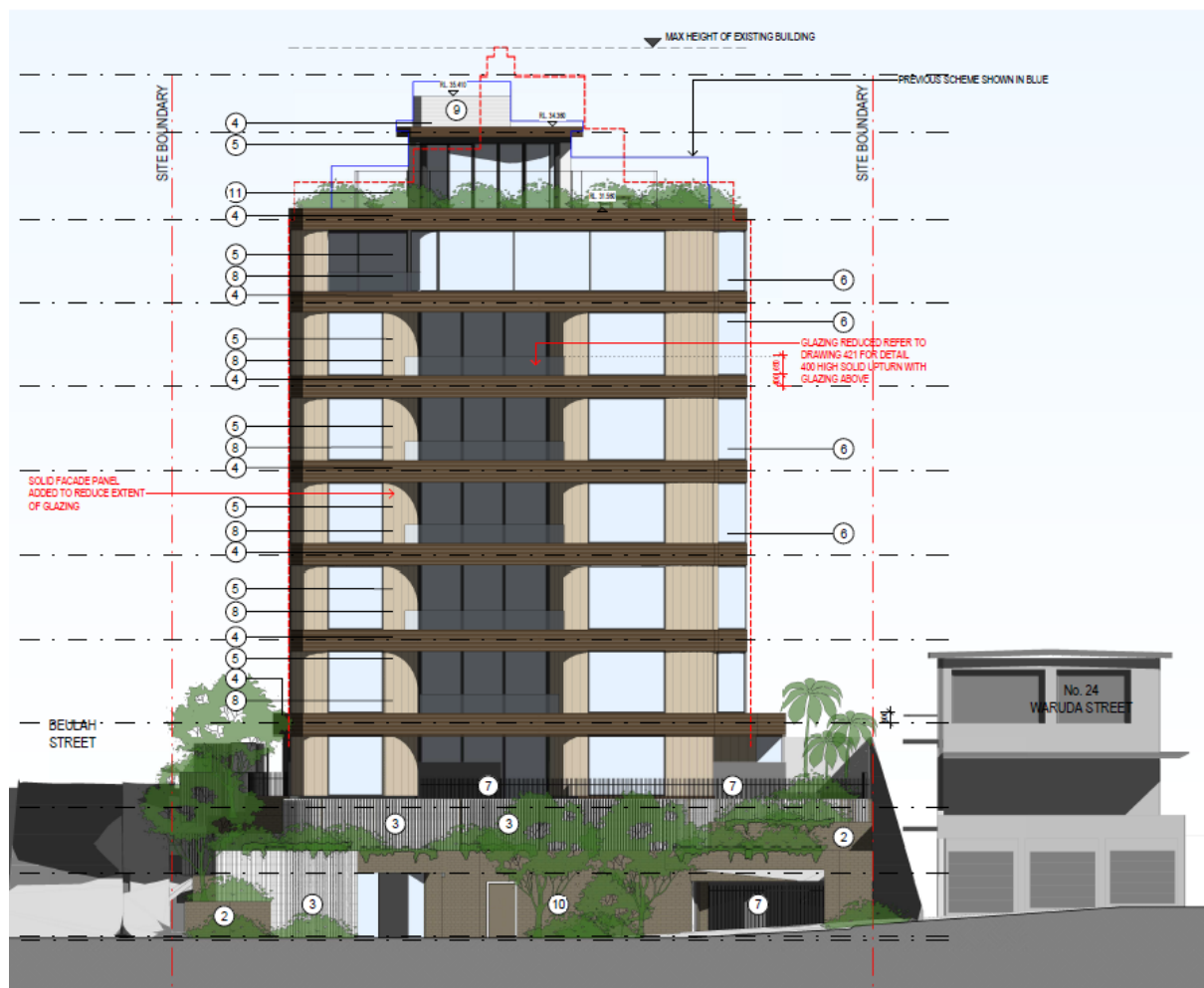
Figure 5: Southern elevation showing pedestrian and vehicular access to the semi basement level from Waruda Street (Nettleton Tribe Architects).
