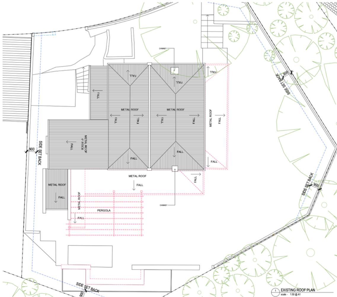
Figure 88.0, Existing Roof Plan and External Demolition, Michael Cumming Architect, 24.02.23
