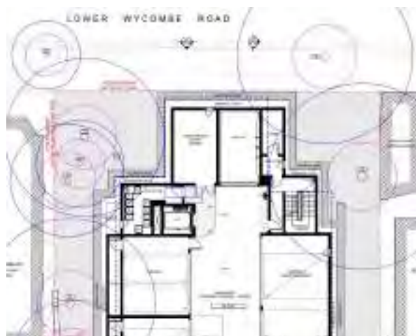
Figure 3: Proposed Basement B1 detailing areas of additional excavation
