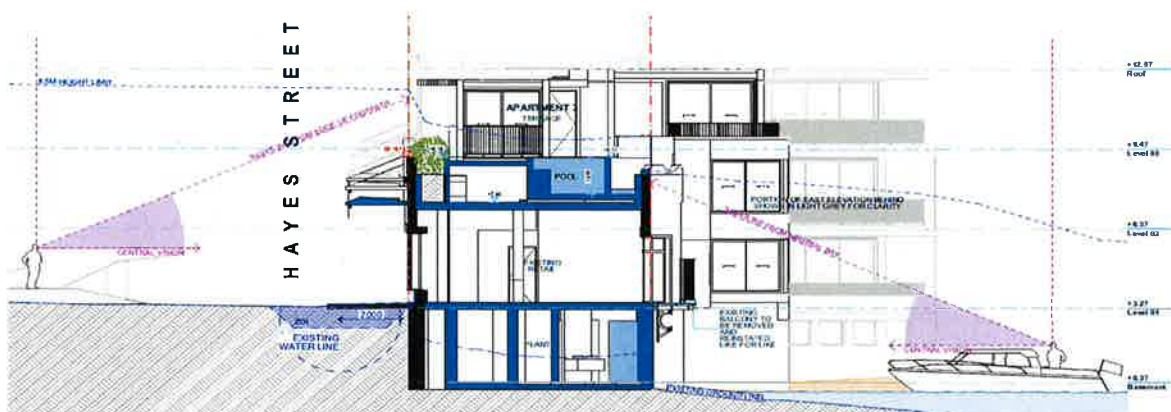
Section showing sight lines from Hayes Street and a vessel adjacent to the Hayes Street Beach (extract of drawing No 117, Popov Bass Architects).
