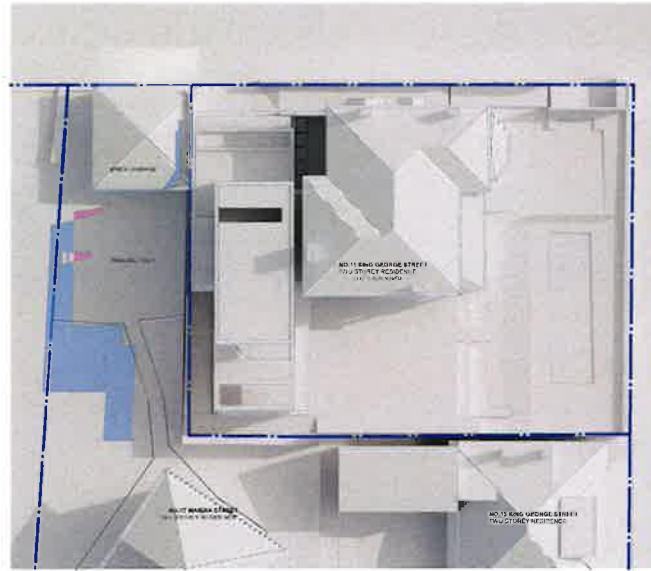
Proposed Shadow Diagram - 21st June 12pm
