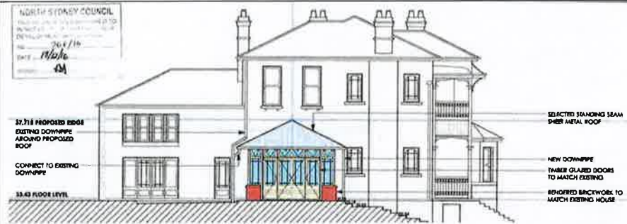
Figure 14 – Approved East Elevation with Conservatory, DA 268/16
