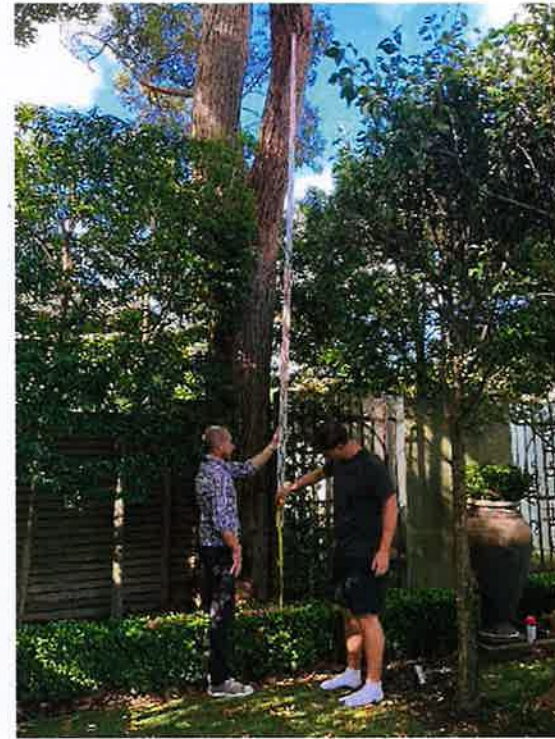
2: Bottom of lowest northern branch confirmed at 5m above grade – 750mm (approx.) of clearance from proposed dwelling addition at closest point
