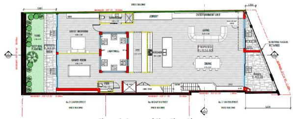
Figure 3: Proposed First Floor Plan
