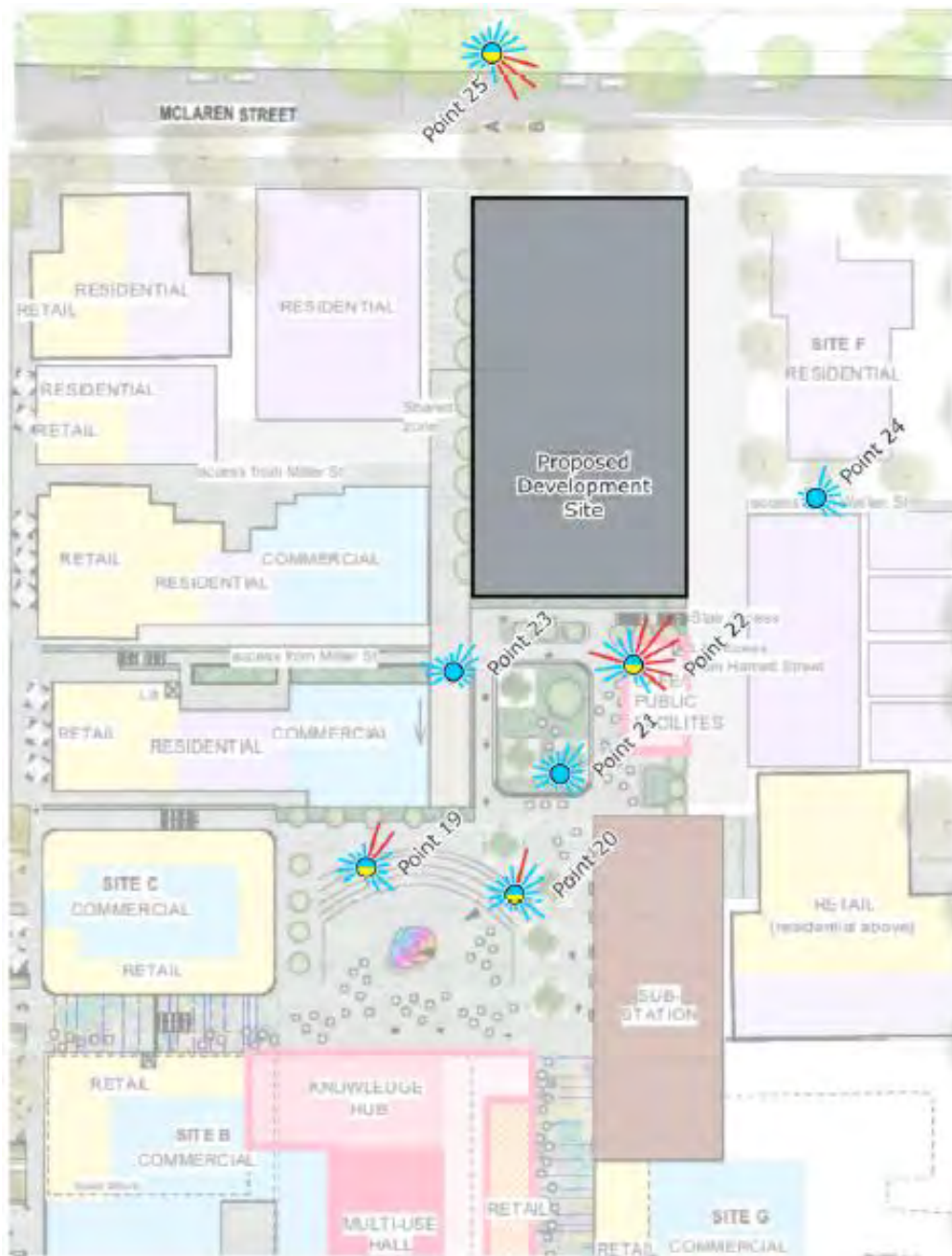
FIGURE 14: Wind tunnel results (Source: Pedestrian Wind Environment Study, Figure 6b)
