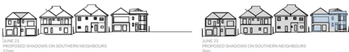
Figure 18. Overshadowing on north-facing façade of neighbours to the south. (Source: Carter Williamson)
