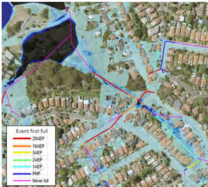
The option was assessed using the TUFLOW model for the 1% and 5% AEP events. The location of the proposed trunk upgrade works and the impact on the 1% AEP flood level is shown Image 40.
