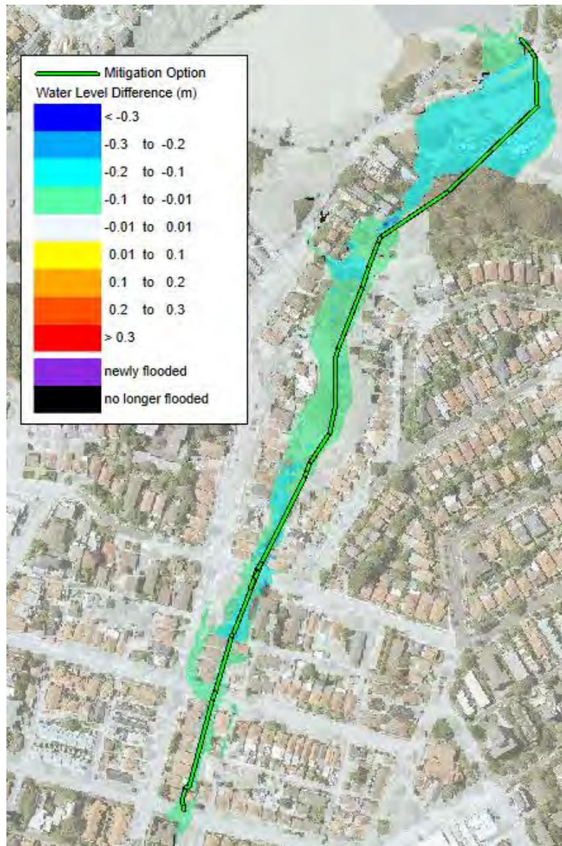
The results show that upgrading the trunk capacity is most beneficial for properties located in proximity to the trunk alignment. With peak flow in the trunk increases from 12.3 m<sup>3</sup>/s under existing conditions to 17.3m<sup>3</sup>/s at the Primrose Park harbour outlet, the 1% AEP peak flood levels decrease by up to 0.05 m on Sutherland Street, 0.22 m on Grasmere Road and 0.21 m on Wonga Road.
