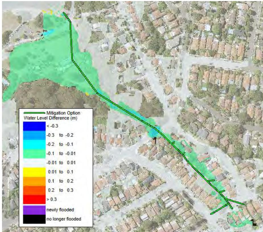
Image 40 shows that upgrading the trunk capacity is most beneficial for properties located in proximity to the trunk alignment. With peak flow in the trunk increases from 12.1 m<sup>3</sup>/s under existing conditions to 15.8 m<sup>3</sup>/s at the Primrose Park outlet, the 1% AEP peak flood levels decrease by up to 0.13 m on Brightmore Street, and 0.15 m on Wonga Road.
