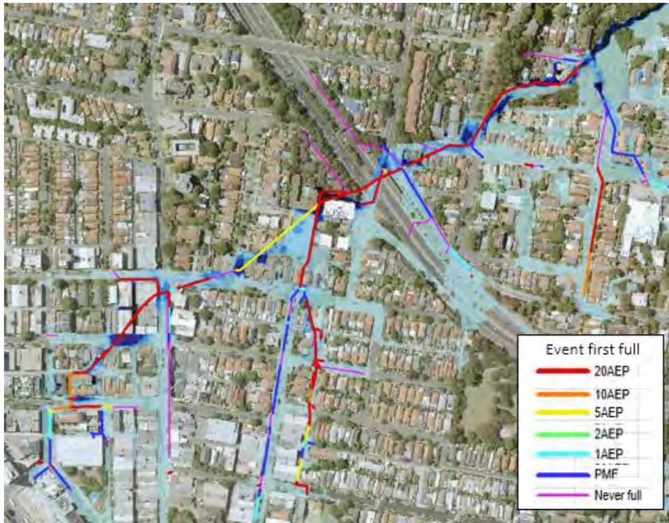
The option was assessed using the TUFLOW model for the 1% and 5% AEP events. The location of the proposed trunk upgrade works and the impact on the 1% AEP flood level is shown in Image 34.
